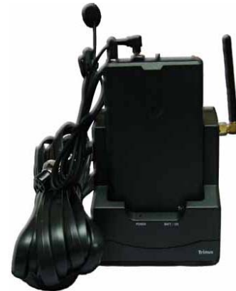
Figure 8 : 900MHz Spread Spectrum Transmitter & Reciever / Charging Base
